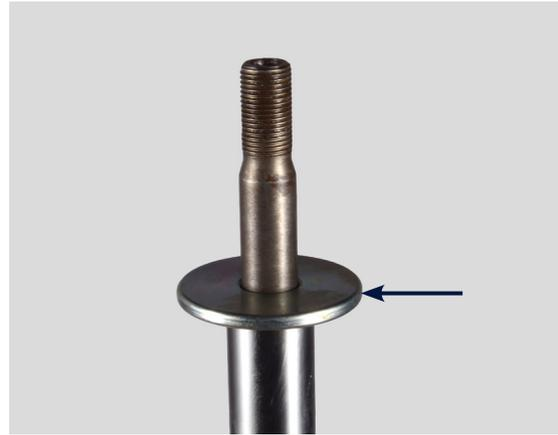
**8.** Place the reaction washer from your kit onto the "shoulder" at the upper end of the shock absorber.
