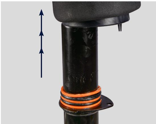
**3.** Gently tap the piston from below using a soft-face mallet in order to lift the piston from its internal seals. Lift-off the air spring bag from the shock absorber.
