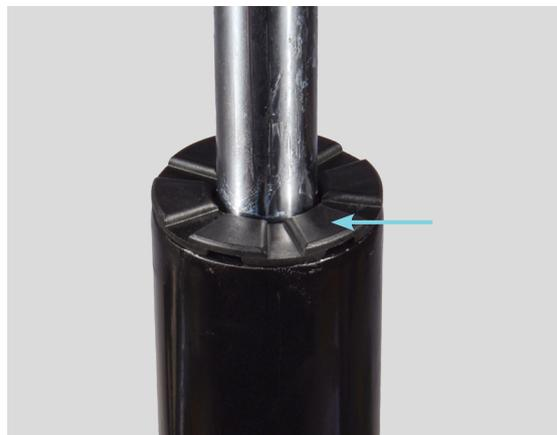
**6.** Place the bump stop lower seat disc from your kit onto the "shoulder" at the upper end of the shock absorber tube, with "teeth" facing upwards as shown.
