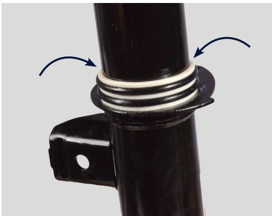
**5.** Place the backup rings (3x) and O-rings (62.0x5.0, 2x) from your kit over the shaft at the top and down onto the piston seat in the silicone-based lubricant to the O-rings.
