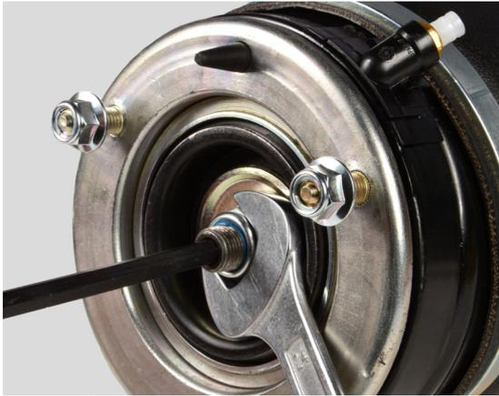
**1.** Remove the nut at the top of the strut: Insert a M8 Allen key into the pin and hold whilst unscrewing the nut using a M24 spanner. Lift-off the washer freed by removal of the nut. Then clamp the strut in a vice at the lower end. Use protective jaws in order to avoid damaging the component.
