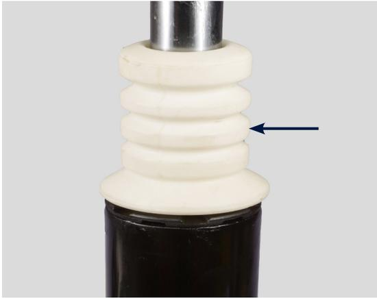
**7.** Place the bump stop from your kit over the neck of the shock absorber and onto the seat.
