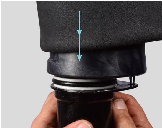
**9.** Place the new air spring bag from your kit onto the shock absorber assembly so that the pin at the base of the piston is inserted into the hole in the piston seat.
