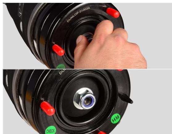
**12.** Install the M16 nyloc nut from your kit: Insert a M8 Allen key into the pin and hold whilst tightening the nut. Ideally use an open-ended torque wrench with a 24 mm fitting and tighten to torque 75 Nm (55lb.ft), otherwise hand-tighten with a 24 mm spanner.
