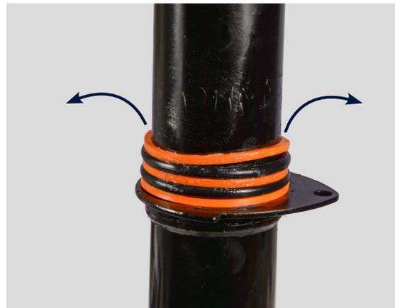
**4.** Remove and discard the existing backup rings (3x) and O-rings (2x).
