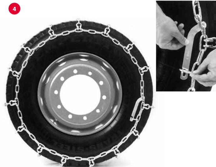
Then tighten the outside chain and close it by means of the tension lever.
