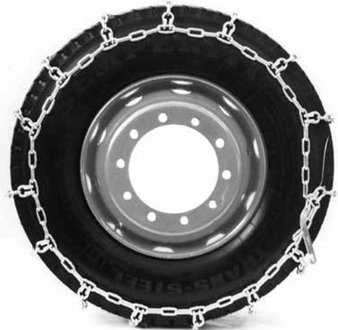
Drive forward one full turn of the wheel, check successful mounting of the chain and remove mounting cable.
