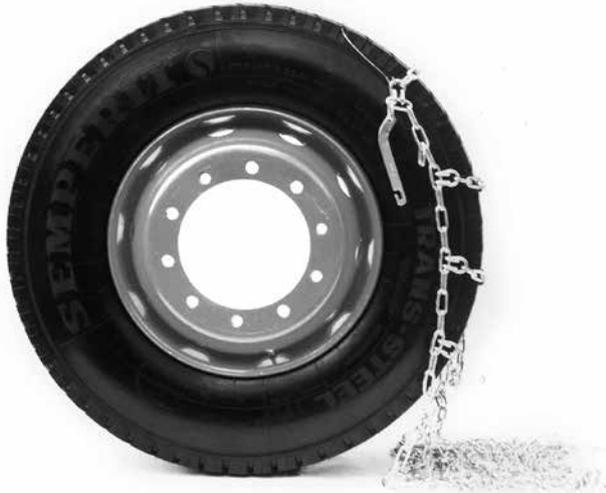
Hang the chain into the tire thread by means of the enclosed mounting cable.
