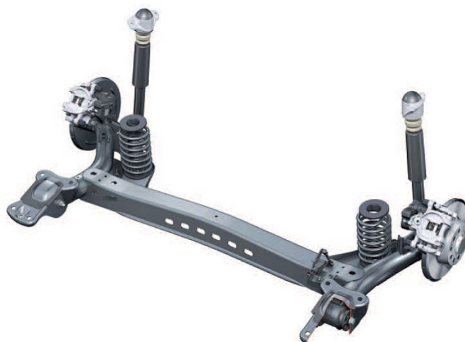
Abb. 2: Verbundlenker-Hinterachse Fig. 2: Twist beam rear axle
