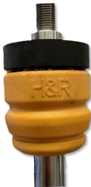
Abb. 2: VA Anschlagpuffer Fig. 2: FA bump rubber
