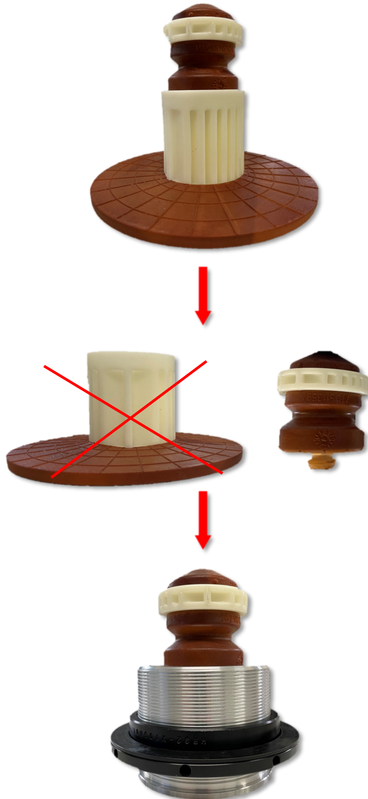
Abb. 4: Montagevorgang HA Anschlagpuffer Fig. 4: Mounting procedure RA bump rubber
