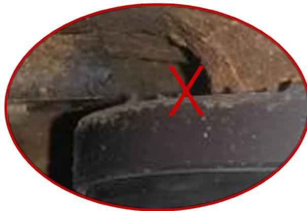
**Solution:** The ABS sensor is being forced away from its correct position by the rust build up behind it on the dust cover plate.
