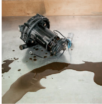
Fig. 28: condensate in the secondary air pump
